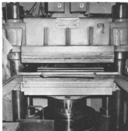
Figure 18. Thermoformed matrix of phenol groups by the Photopolymer Plate
